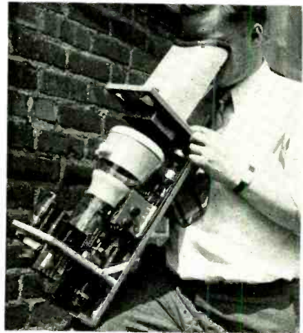
Electronic view-finder with cover removed. Note the special squatty cathode-ray tube employed
