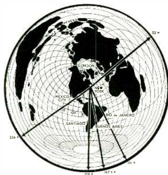
Fig. 2—Azimuth chart of the world centered on New York. The same antenna (with radiator and reflector interchanged) may be used for transmission to London or Mexico City
