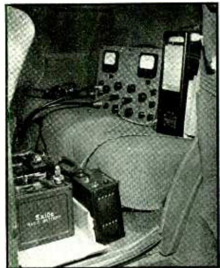
Fig. 3—View of the equipment used in field-intensity surveys of W2XOY. Note the automatic recorder
