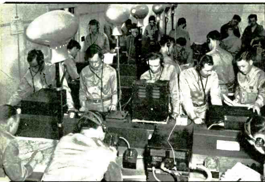
A laboratory class in radio compass work. A complete radio transmitter and receiver are available at each bench position. The line of dirigibles at the left are a group of "tear drop" loop antennas
