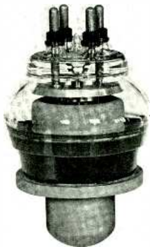
Exterior and x-ray views of the General Electric type GL-880 phototube. Alignment of the internal structure can be checked by the use of x-rays
