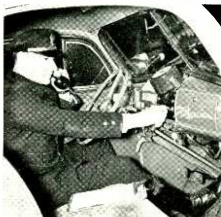
Interior of radio patrol car used to dispatch trolleys and buses
