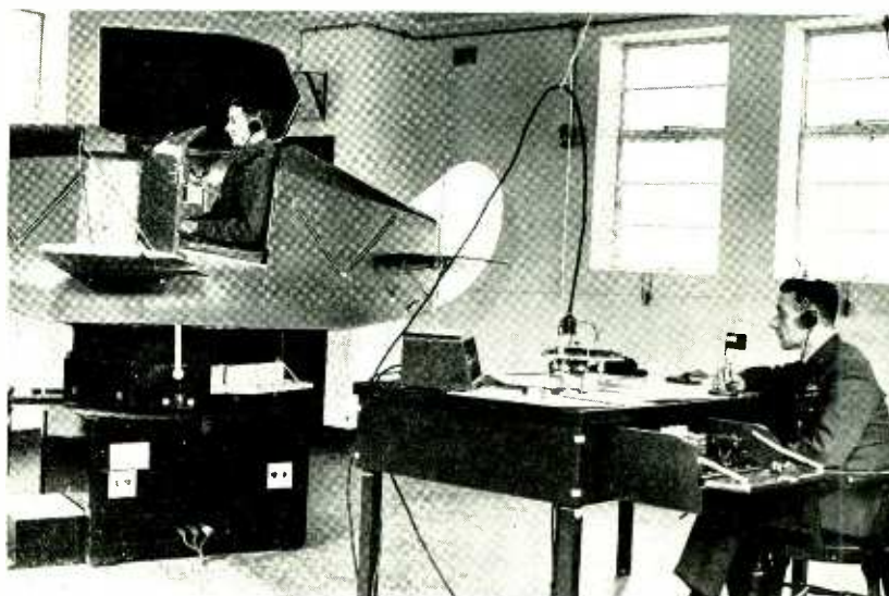
In England, cooperation between the Army and the R.A.F. is highly organized. The man at the desk is an R.A.F. instructor, who is assisting in the training of an Army pilot in the Link trainer which simulates actual conditions of flight even though the pilot and his craft do not leave the ground
